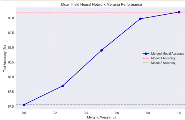
Figure 15: Test accuracy vs merging weight \alpha for the two-model MFNN merge. Dashed lines: individual models.
